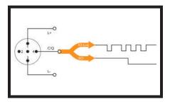
The 0942 UEM 620 I/O-Link master module provides point-to-point connections for the intelligent sensors and actuators by means of the I/O-Link protocol. The four ports can be configured as digital I/Os or for communications mode.
