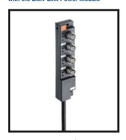
The LioN-Link 0941 UNC 601/...M power module is used for decentralized power supply for I/O modules. It has four ports, two potential circuits and a 10 m lead with a conductor gauge of 5x1 mm². This provides for bridging distances of up to 25 m without voltage loss as well as for configuring separate potential groups each with their own fuses.
